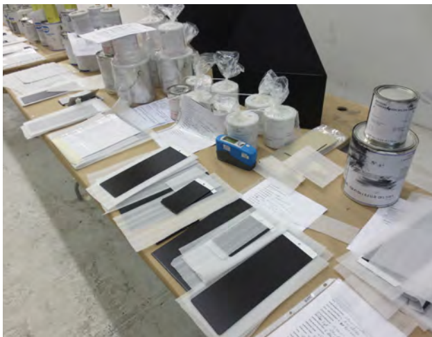
Figure 7 Various black paints are compared to help determine the most appropriate paint for a Tony Smith sculpture. Such comparisons call on the expertise not only of paint manufacturers and applicators but also of conservators and artist's estates.
