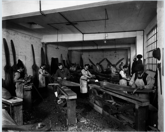
Men and women shaping wooden propeller blades for military aircraft at the factory of construction company Dove Brothers Limited, in Cloudeley Place, Islington (1918; BL24379/003). Reproduced by permission of English Heritage
