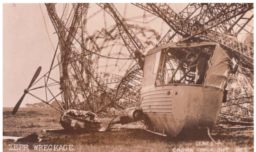
The wreckage of Zeppelin L33, brought down at Little Wigborough, Essex, in September 1916. Photo courtesy of David Marks
