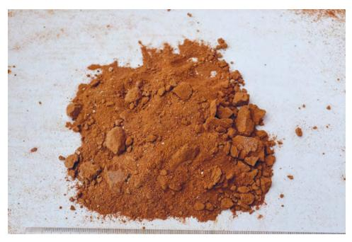
Fig. 6 Old clay mortar is often soft and can be easily broken down.
