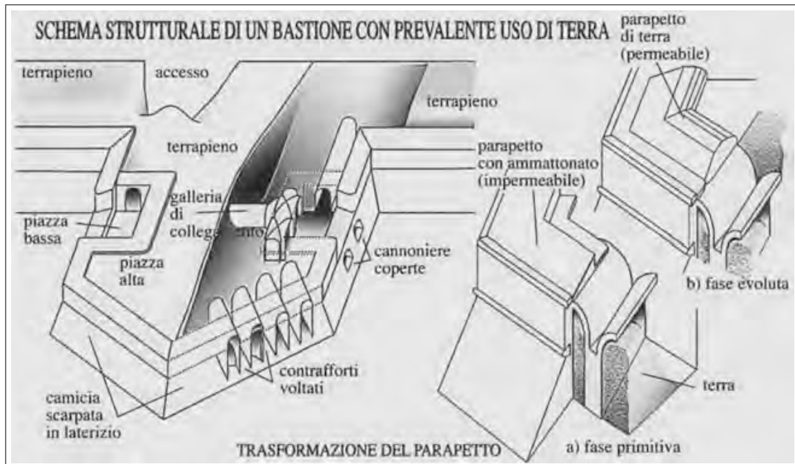
Figure 4.19.: A schematic reconstruction of a bastion according to the concepts of military engineering in the 3rd/4th decades of the 16th century [M. B., 1995].
