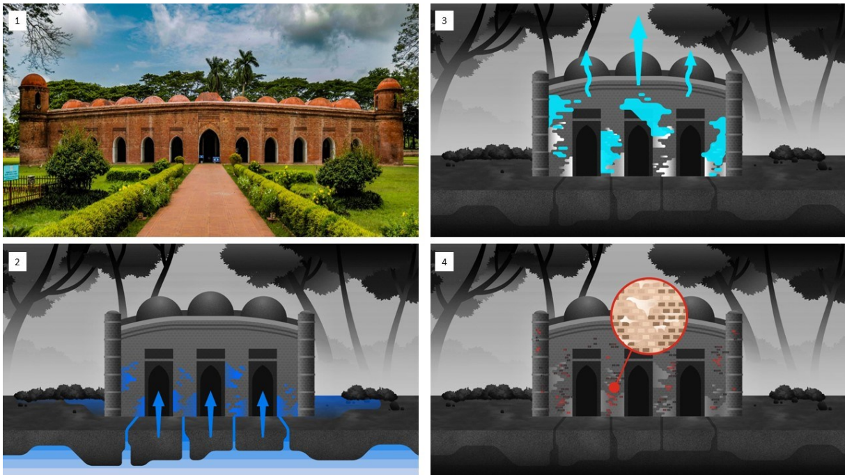
Figure 4. Efflorescence at the Historic Mosque City of Bagerhat. 1) The Sixty Dome Mosque, 2) Infographic showing rising saltwater permeation into brick masonry, 3) Infographic showing water evaporation from structure and, 4) salt on brick masonry © Images from Google Arts and Culture, 2021
