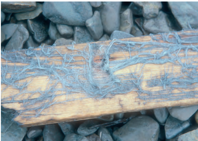
Defibrillation of wood surfaces was found on some woods at Beechey Island and at Fort Conger. Salt accumulation is responsible for causing a chemical attack on wood that results in the separation and detachment of wood cells. Loose surface wood fibers are eroded off exposing new cells to the corrosive action of the salts. Both photos: R.A. Blanchette
