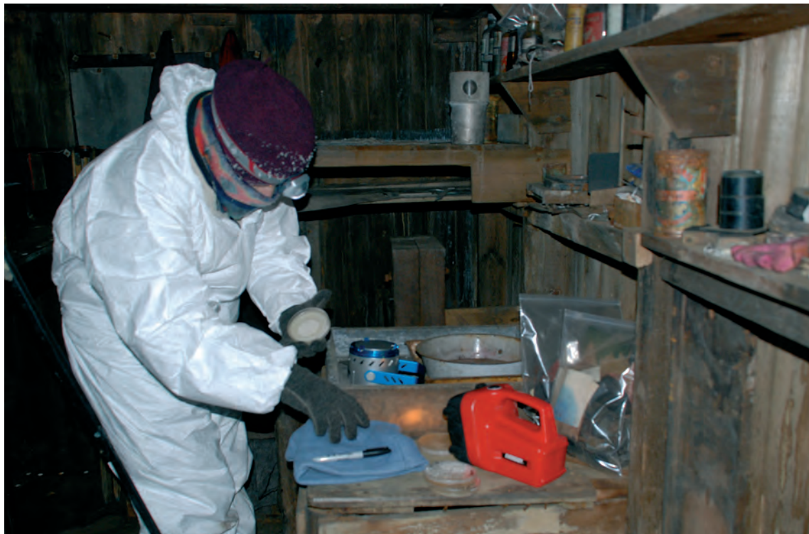
Fig. 4: Testing for aerial spores using a Merck MAS-100 Eco® in Terra Nova Hut, August 2007. Photo: Phillipa Barn.
