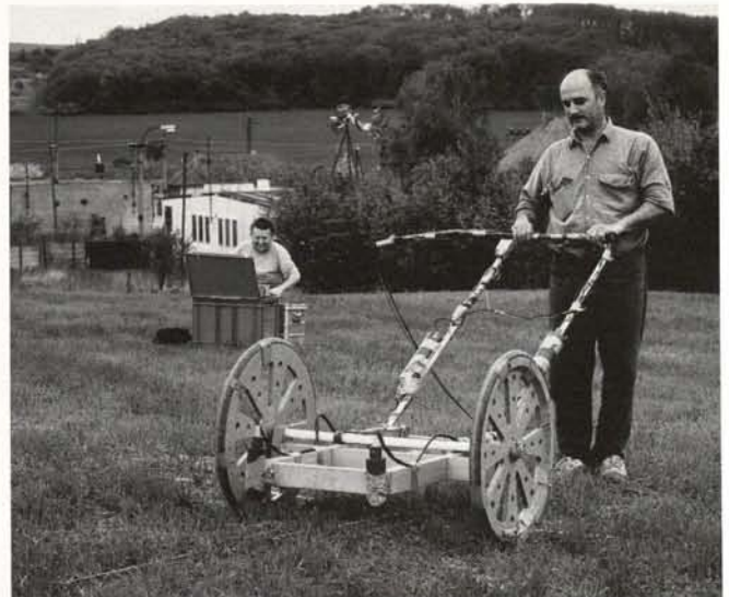
Fig. 2. Magnetic prospection with a Scintrex CS2 caesium magnetometer with the duo sensor configuration
