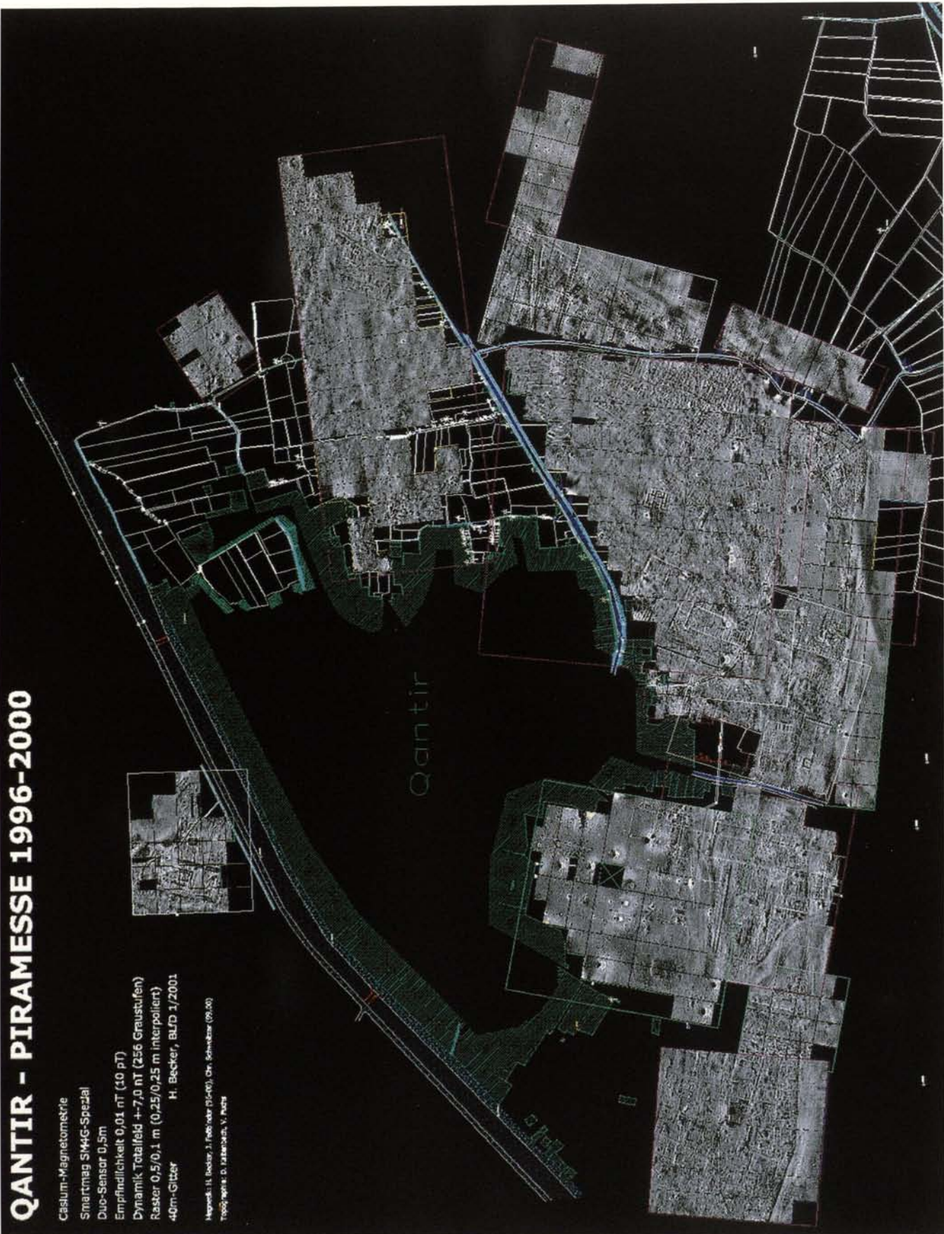
Fig. 4. Qantir-Piramesse. Compilation of the magnetograms from 1996 to 2000 on the topographic map. SMARTMAG SM4G-Special as duo-sensor. Sensitivity 0.01 nT (10 picotesla), raster 0.1/0.5 m interpolated to 0.25/0.25 m, dynamics -7.0/+7.0 nT in 256 gray scales (black/white), mean value between original data and high pass filter, 40 m grid, magnetometer prospecting H. Becker and J. Faßbinder (1996-2000), Chr. Schweitzer (1999, 2000), topography V. Fuchs, D. Kaltenbach.
