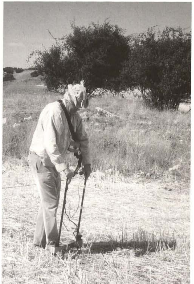
Fig. 1b. Ambrona-Dolmen de la Sima 1998. Resistivity survey using Geoscan RM15-Advanced Resistance meter with twin electrode
