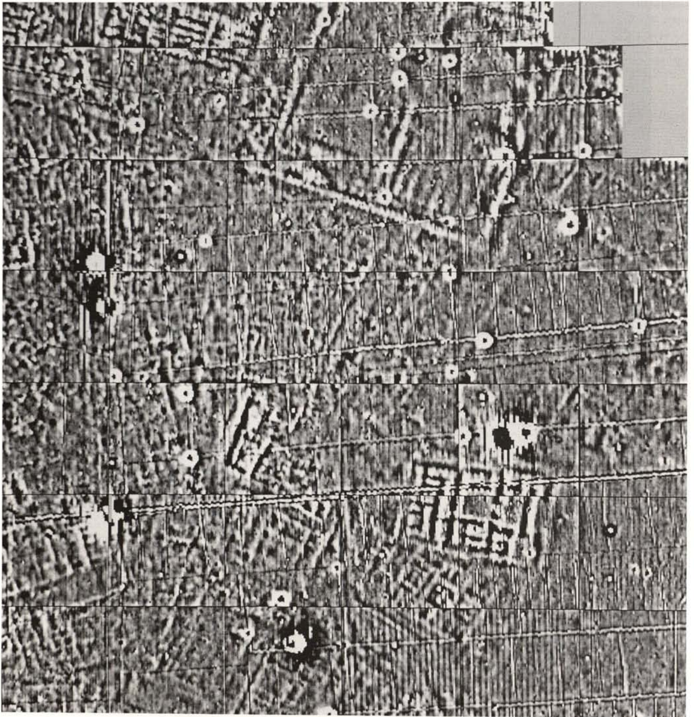
Fig. 5. Qantir-Pirameses East 1997/1998. Magnetogram of the same data as fig. 4, but highpass filtered data 10 x 5 pixel, technical data see Fig. 3a, 3b
