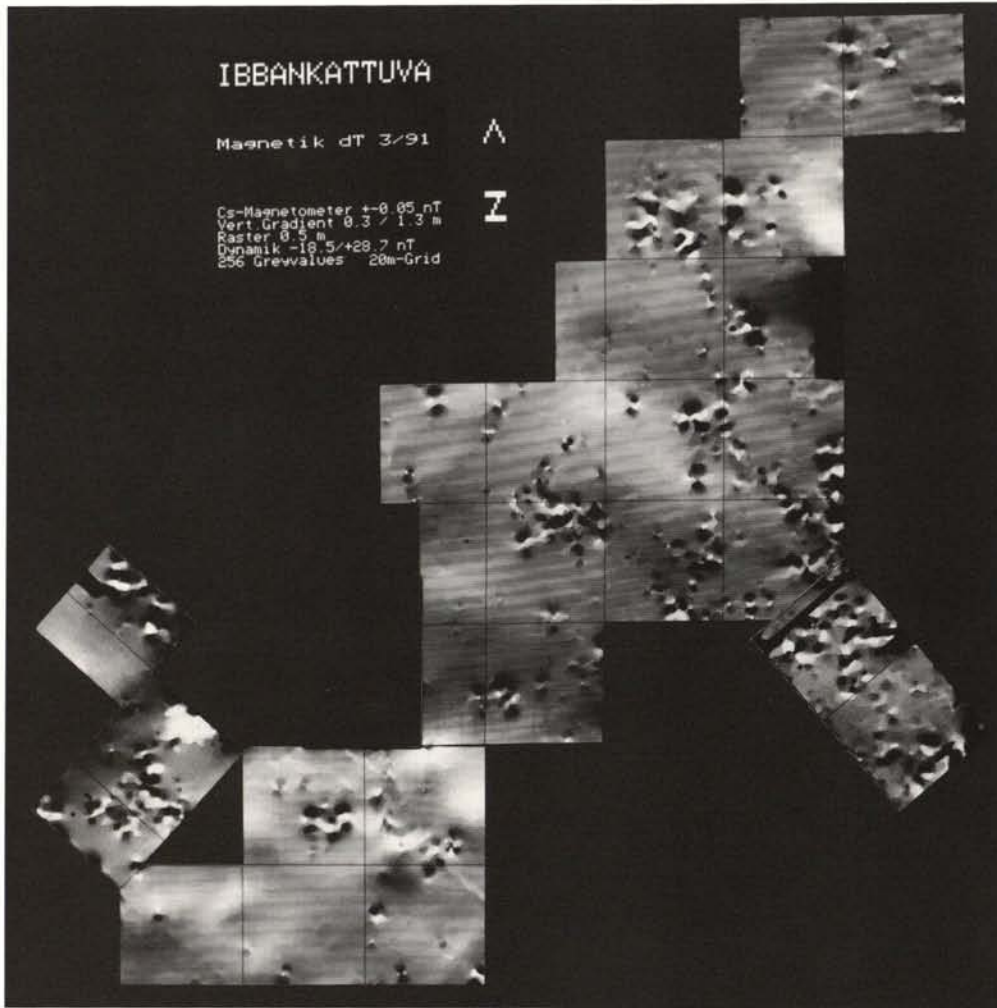
Fig. 3. Ibbankattuwa. Digital image of the magnetometer data of the surveyed area at Ibbankattuwa. Magnetogram in the digital image processing technique. Caesium magnetometer system from Varian/Scintrex, V101, Canada, sensitivity \pm 0.1 Nano-tesla, gradiometer configuration, dynamics -10.0 to +15.0 Nano-tesla in 256 grayscales, sampling rate 0.5 meter, grid 20 x 20 meter
