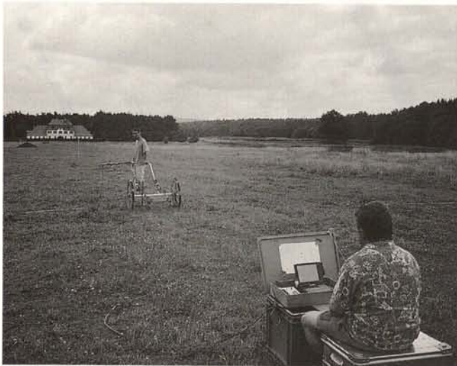
Fig. 2a, b. Duo-sensor on wheels with CS2/MEP720 system (application at Seehof, Photo J. W. E. Fassbinder) and one man carried SMARTMAG SM4G-Special (H. Becker in Resafa 1999, first use by H. Becker at Monte da Ponte in 1995)
