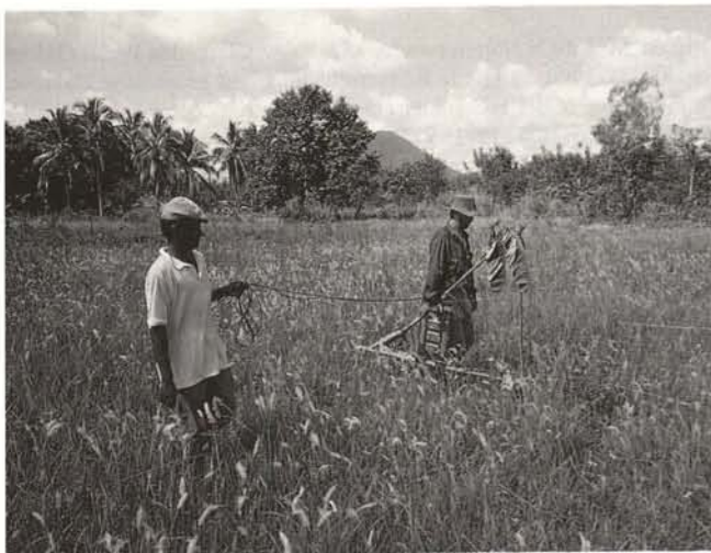
Fig. 2. Ibbankatuwa. Caesium magnetometer system employed in Sri Lanka. The probes are covered by banana leaves to give them a shelter upon the sun. The caesium magnetometer with vertical gradient configuration of the sensors; difficult to see: the tilting of the probes by proximately 45° to the north direction
