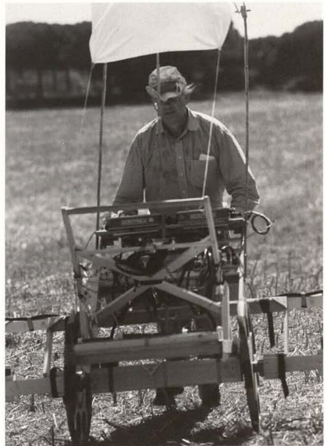
Fig. 1. "Magneto-Scanner" of the Bavarian State Authorities for Monument Conservation at its first test in Ostia Antica 1996, consisting of four caesium magnetometers Scintrex SMARTMAG SM4G-Special with quadro-sensor configuration, two gradiometer consoles-data loggers, power supply (4 batteries 12V/6Ah) and automatic distance trigger mounted on a nonmagnetic chariot, total weight about 50 kg), proto-type 1996
