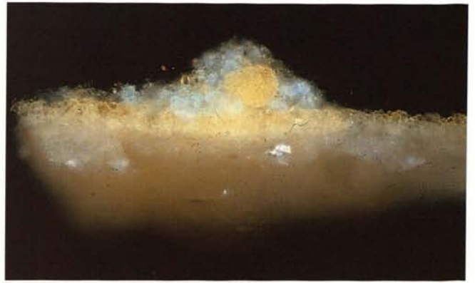
2: Cross section of a woman's carnation sampled from the Akhetetep's mastaba (Louvre E 10958): 1-stone, 2-ground layer made of calcium sulphate, 3-yellow layer composed of pigments from the "jarosite minerals group", 4-copper chloride and calcium sulphate, © LRMF, S. Colinart.
