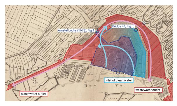
^ Fig. 4 Flushing scheme in the second half of the seventeenth century until 1872. The blue arrows indicate the clean inlet water, and the red arrows indicate wastewater-enriched outflow. Locations of fig.1 and 5 are indicated. (Source: Map: Stadsarchief Amsterdam, KOKA00125000001).
