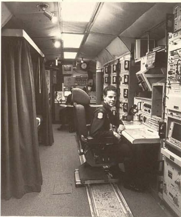
Fig. 5. The operational center of the Minuteman missile system was the underground Launch Control Center. Here two man missile crews were stationed 24 hours every day of the year and could be alerted to launch 10 remote nuclear-tipped Minuteman missiles.
