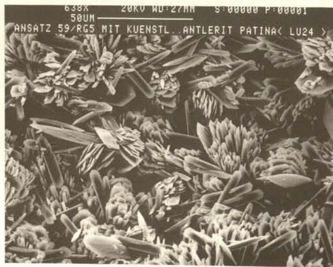
Fig. 7. SEM micrograph: artificial antlerite on Rg5 alloy
