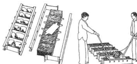
(Fig. 1) Filling the mould with rubble stones and compacting.
