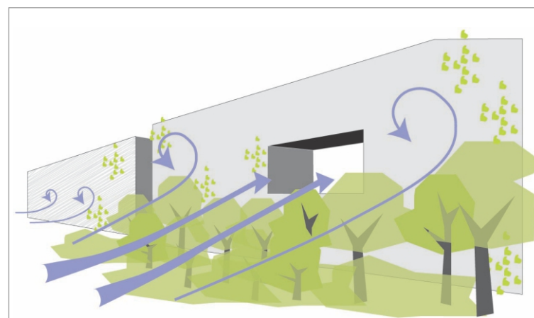
Open building design for better ventilation/air circulation in dense urban areas.
