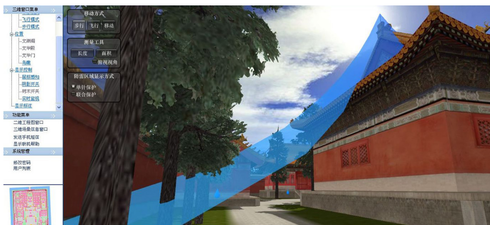
Figure 9. Simulation showing a gap in coverage on the trees at the Hall of Literary Brilliance
