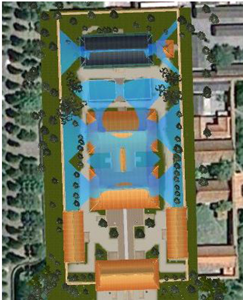
Figure 10. 3D virtual top view of the comprehensive protection coverage of lightning protection devices at Hall of Literary Brilliance
