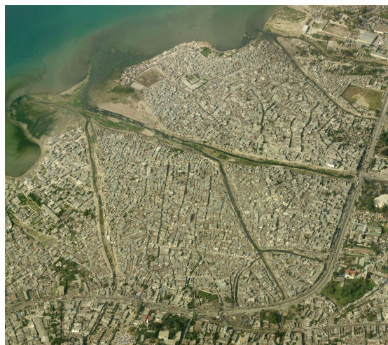
Figure 15. 3D aerial view of shanty town on the hills immediately to the south of Port-au-Prince city centre. One can see that only occasional houses on the less steep areas are collapsed, but massive slides and collapses are along the steep slopes of the ravine. The 3D image made from Pictometry images with overlapping sections (To view in 3D, cross your eyes until so that you can see the two images exactly overlap) (© Pictometry).
