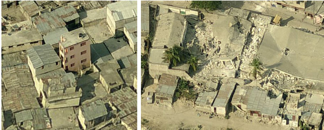
Figure 17. Left: Typical detail of 'Cité Éternelle' showing that two story buildings with one four story building, most of which are constructed using reinforced concrete
