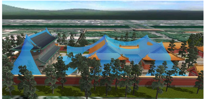
Figure 8. Brilliance 3D simulation schematic diagram II of comprehensive protection scope of lightning protection devices at the Hall of Literary Brilliance
