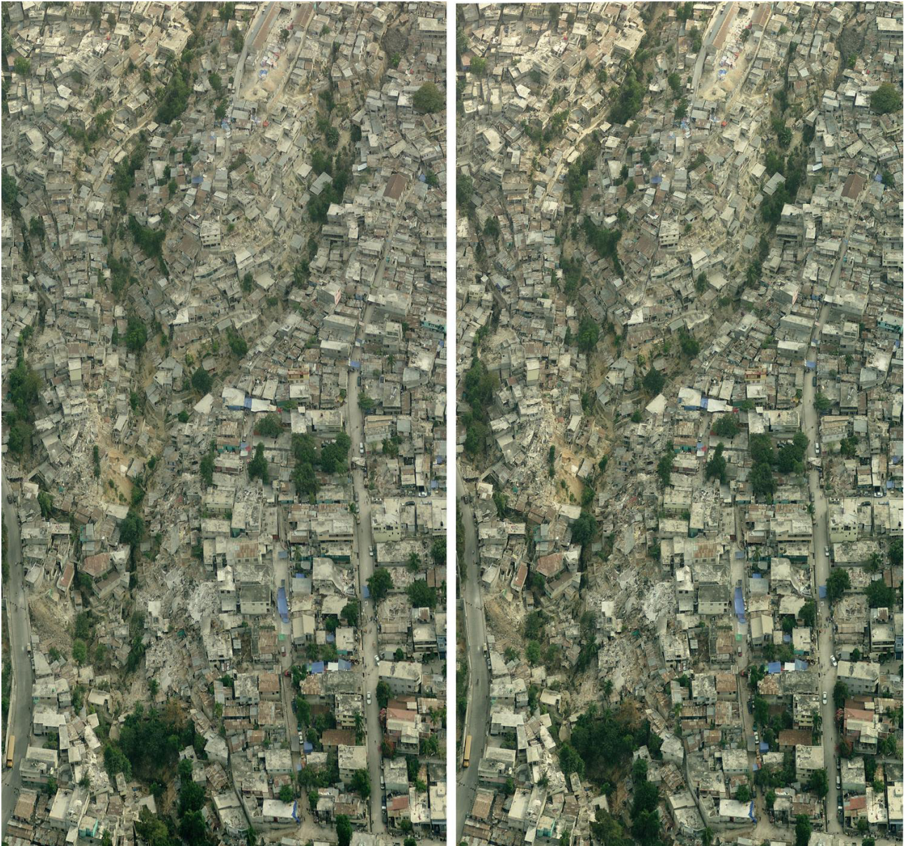
Figure 15. 3D aerial view of shanty town on the hills immediately to the south of Port-au-Prince city centre. One can see that only occasional houses on the less steep areas are collapsed, but massive slides and collapses are along the steep slopes of the ravine. The 3D image made from Pictometry images with overlapping sections (To view in 3D, cross your eyes until so that you can see the two images exactly overlap) (© Pictometry).
