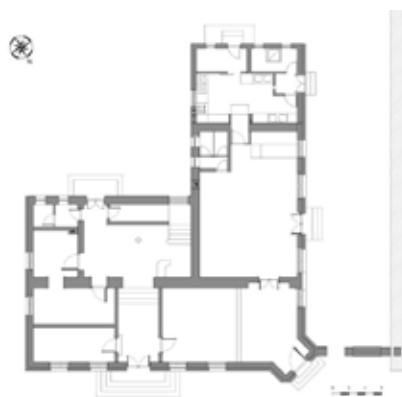
Drawing 2. Plan of the ground-floor, new condition
