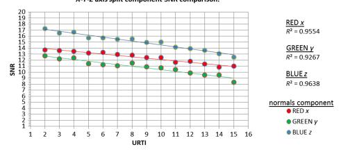
Fig. 21 SNR in the three geometric axis of URTI surface normal renders under varied turbidity.
