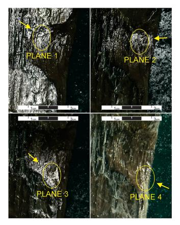
Fig. 14 Illustration demonstrating relighting the URTI produces four distinct planes of "mirror-like" reflection under specular enhancement.
