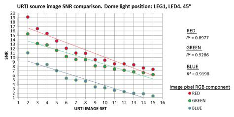
Fig. 19 SNR in 45-deg tier URTI source photos under varied turbidity.
