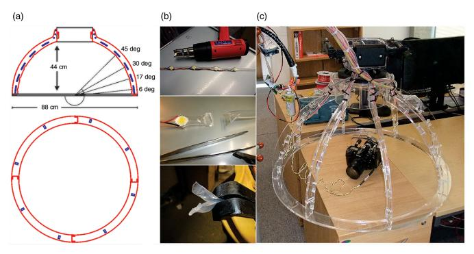
Fig. 3 (a) Dome CAD drawing, (b) heat-shrink wrapping of dome LED electronics, and (c) the completed dome featuring Nikon D300 camera.
