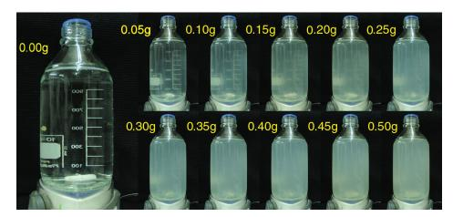
Fig. 11 Illustration of the change in turbidity induced on 1 I of fresh water by the progressive addition of bentonite clay.
