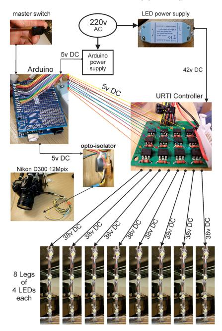
Fig. 4 Dome electronics flow chart pictorial.
