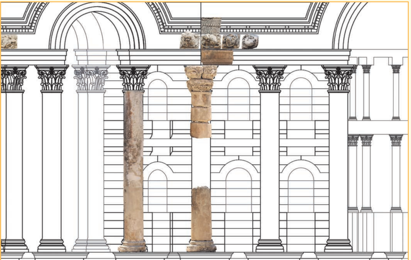
Figure 45: A computer generated drawing showing the location of the previous column with anastylosis. This drawing was used in one of the signs at the site
