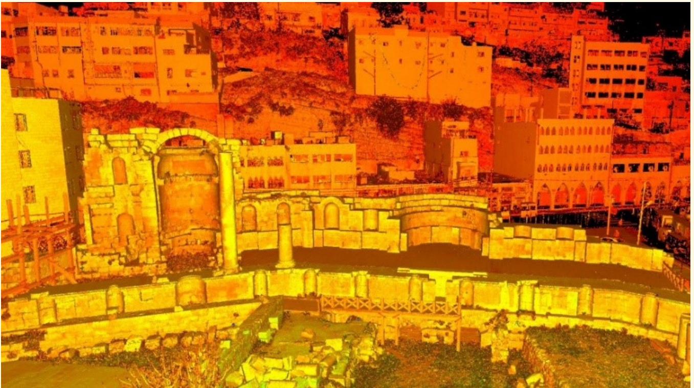
Figs. 64: A view of a point cloud image for the main façade from the 3D scanning of the Nymphaeum
