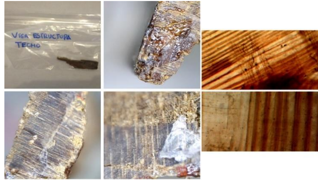
Fig.3. Wood of structure of the house ( Pinus Strobus L. ) (Carreras, 2019)
