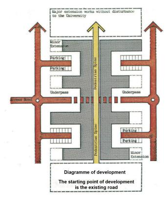
**Fig. 6. Diagramme of development.** Linear development, along a pedestrian spine, allows the most flexible form of urban development ("stop and go"). In the case of Louvain the initial development started from the existing N4 road and extended along the spine from east to west, an adaptation of the linear development designed by G. Epstein in 1964 for the University of Lancaster (EPSTEIN 2009)
