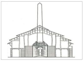
3-a Plan 3-b. The section of the kiln
