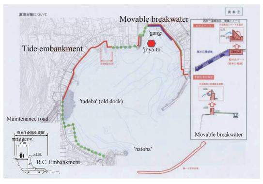
Fig. 13. Construction Plan of Tide embankment&Movable breakwater, 2015& Distribution of historic port facilities-'gangi', 'joya-to', 'hatoba', 'tadeba'.
