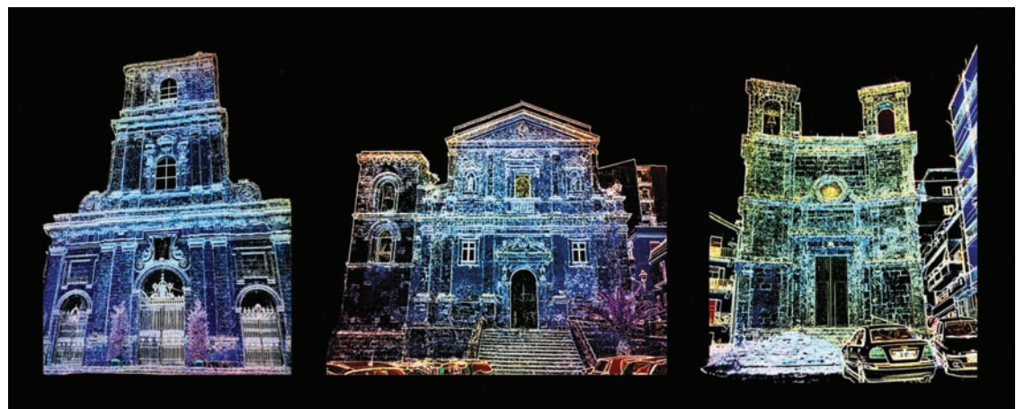
Fig 03 Filtered images to overlap to the point cloud, Churches of Enna
