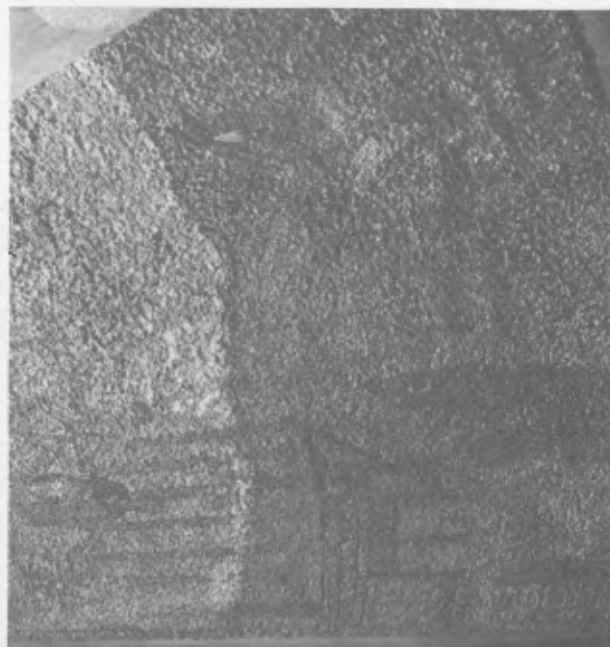
Fig. 7 - The reverse side of a mosaic, cleaned by an ultrasonic chisel. The design on its other side is clearly visible
