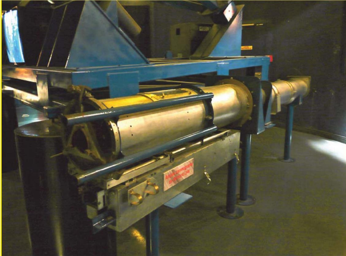
**Fig. 9.14.** The first coronagraph in the world. Invented and tested by Bernard Lyot at the Pic du Midi. It is displayed in the museographic space in the observatory (2013). Photo © Régie du Pic du Midi and Observatoire Midi Pyrénées
