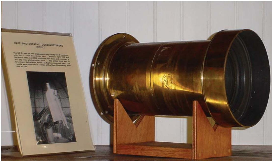
**Fig. 8.8.** Dallmeyer Portrait lens (1880s) used for making the Cape Photographic Durchmusterung, the first photographic sky survey. Photograph © Ian Glass
