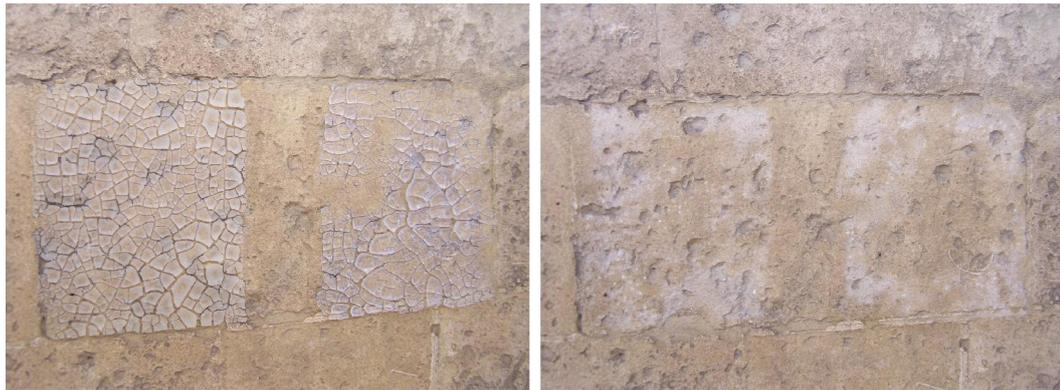
Fig. 7. In situ biocleaning test performed on the lateral wall of Matera cathedral; laponite biogel bacteria, after 48 h of bioapplication, before (left) and after (right) the soft biogel removal.
