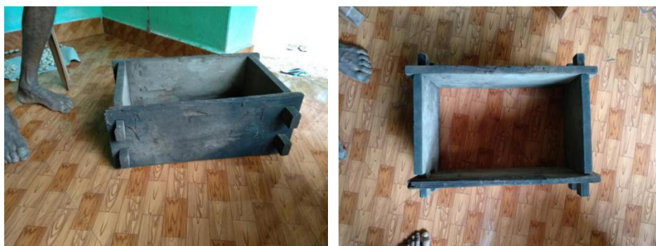
Image 77 and Image 78: Mason Babuso's adobe-brick mould.
