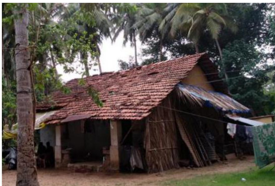
Image 133: Palm-leaf barriers poised parallel to earthen walls protected the walls from rainwater (Survey no. 1).
