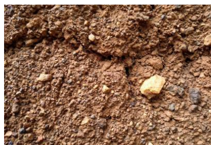
Image 80: Yellowish soil; includes clay, sand, and rubble (Survey no. 4).
