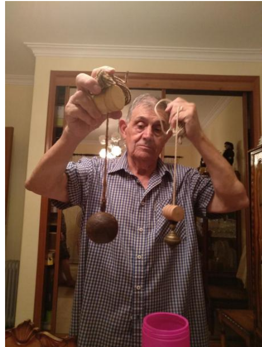
Mason-Sailor Joaquim showing his 100 years old plum tool used in rammed-earth constructions.
