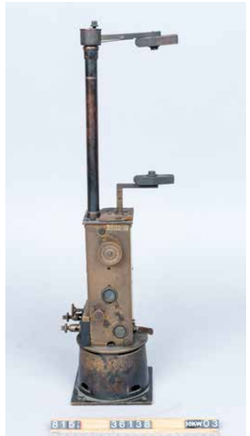
Abb. 6: Bogenlampe, Siemens & Halske, System Hefner-Alteneck (Inv.-Nr. 36138)
