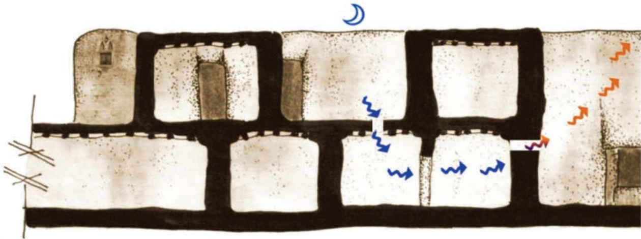
Fig. 3 Cross section of one of the houses explains night cooling using “night flush-out”. Cool outdoor air is introduced into the building at night to allow the interior to pre-cool for the next day. Occupants have to open and close windows when needed. It is most effective as thermal mass helps store cool air for the next day.
