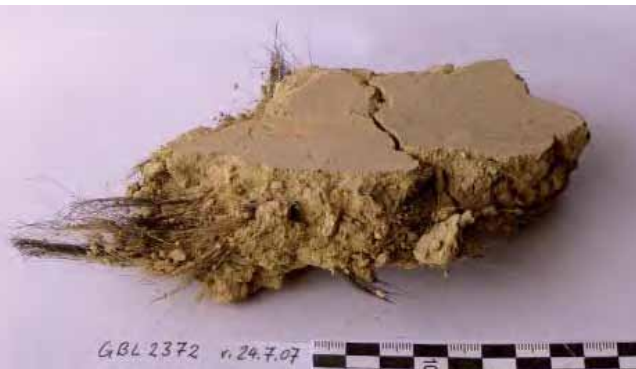
Fig. 21. Hair, sometimes in tufts, in the undercoat of the Western Buddha [Melzl]
