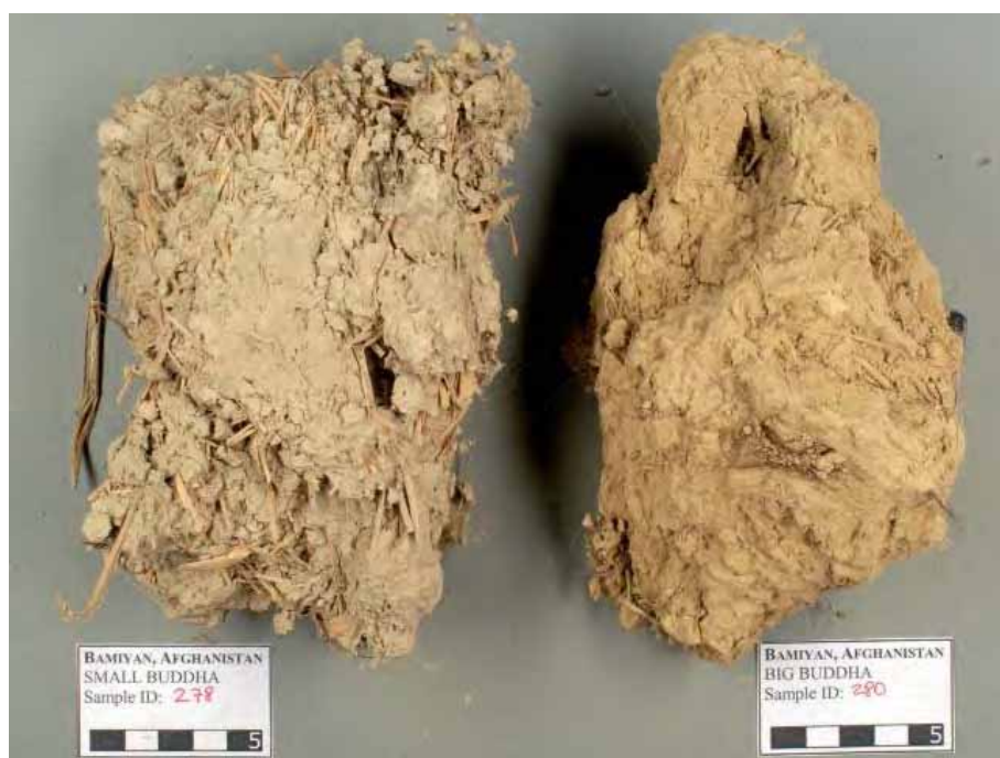
Fig. 1. Loam plaster fragments of the Eastern Buddha (sample 278, left) and the Western Buddha (sample 280, right) [Höfle, Thiemann]
