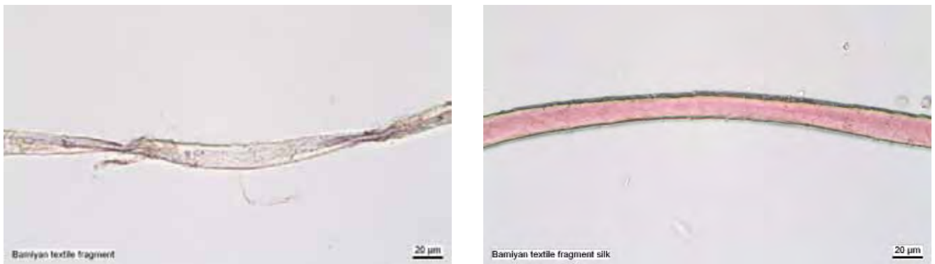
Fig. 6. Fibres of textile in transmitted light: cotton (left), red-dyed silk (right)
