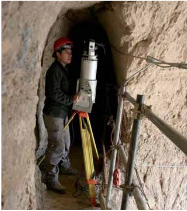
Riegl Laser Scan Z420i in various scan positions
