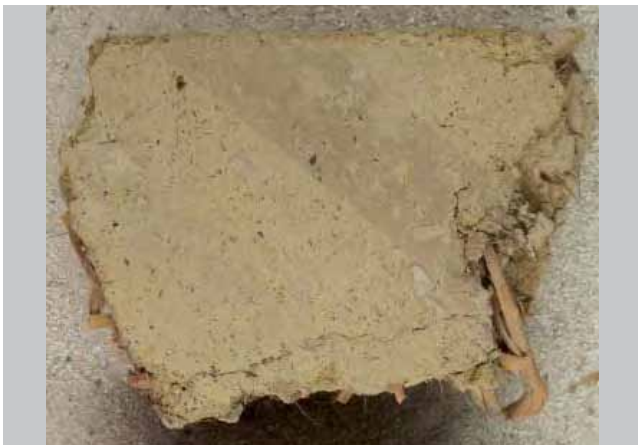
Fig. 19. Sample ID 67 from Western Buddha; trace of a 15 mm wide line preserved in the isolation layer (paint layer missing), length of fragment 40 mm
