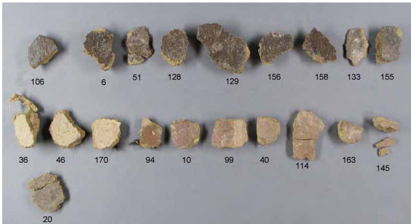
Fig. 8. Western Buddha, group 3: Samples with glossy, structured surface (top row), matt surface (middle row) and white below brown (lowest row)
