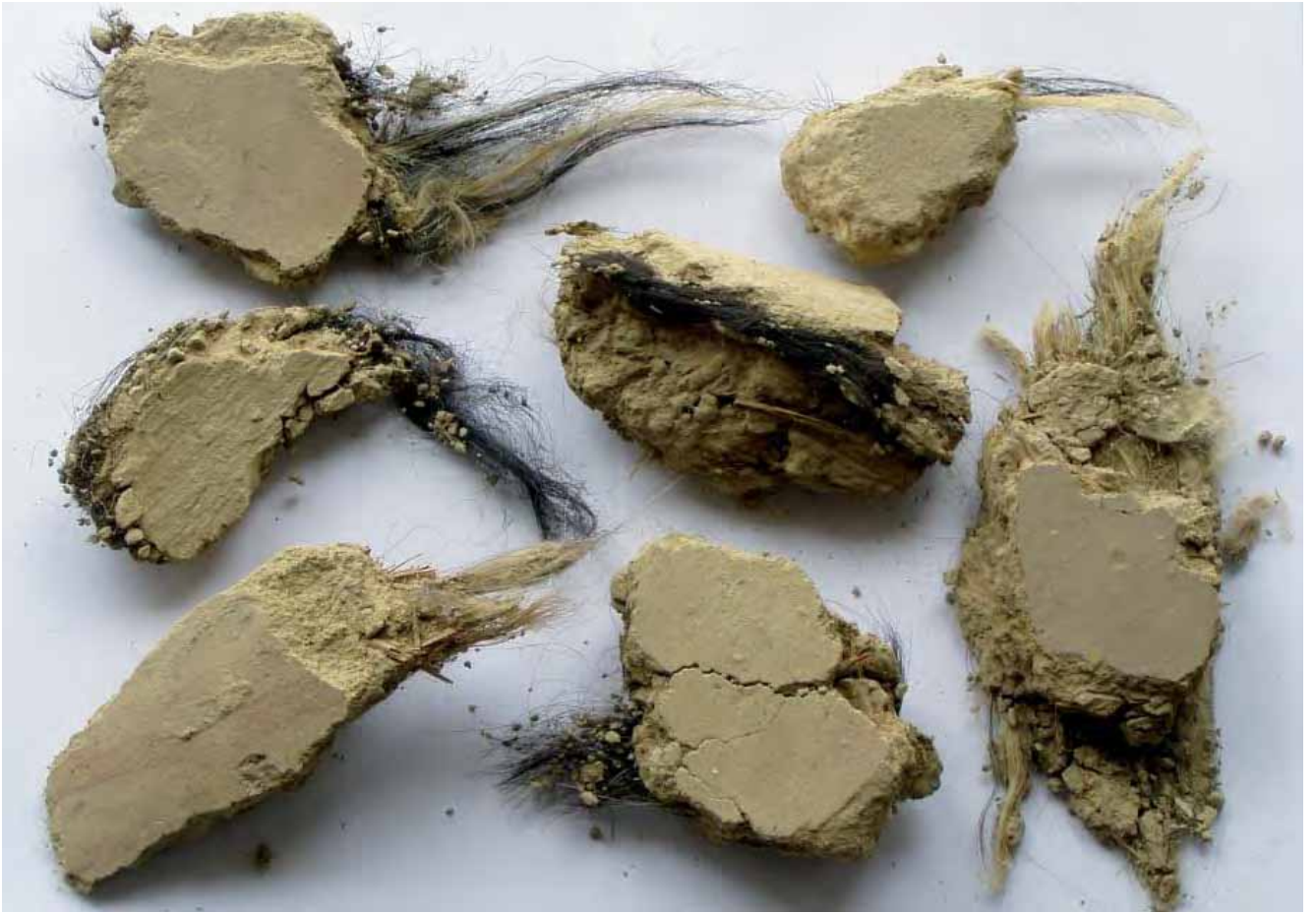
Fig. 1. Fragments GBL 2377-2833 from the Western Buddha containing large amounts of hair [E. Melzl]
