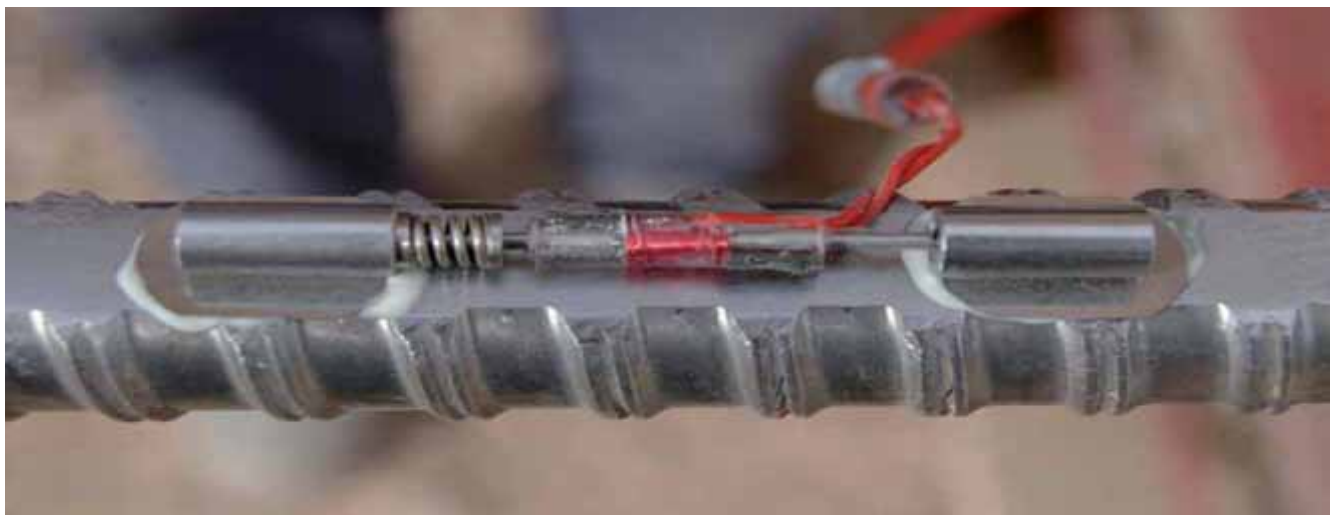
Fig. 31. Detail of a strain gauge
