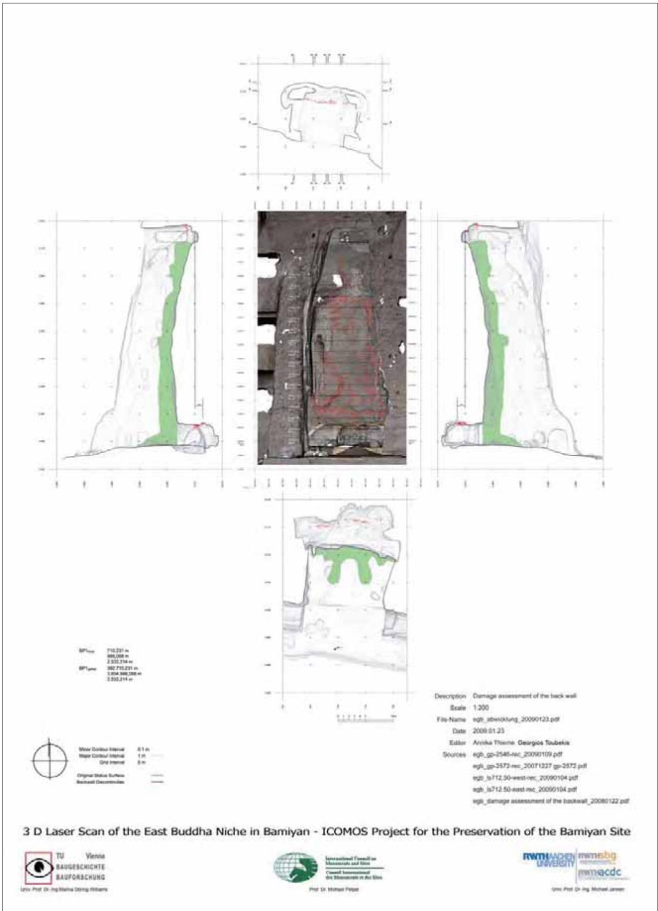
Fig. 12. 3D laser scan, damage assessment of the back wall with original statue surface (green), back wall discontinuities (red)
