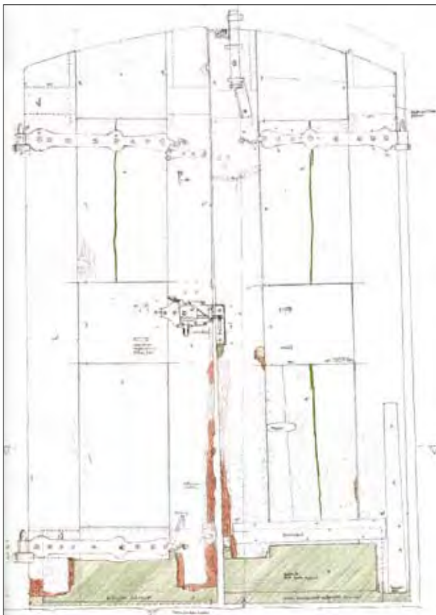
◁ Damage map of a door from the former monastery of Thierhaupten, exterior and interior view (drawing: Martim Saar)
