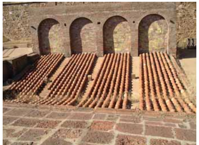
Fig 8 Aludel or Bustamante furnaces on display in Almadén
